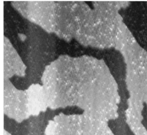
3x1 reconstructed GaAs surface
